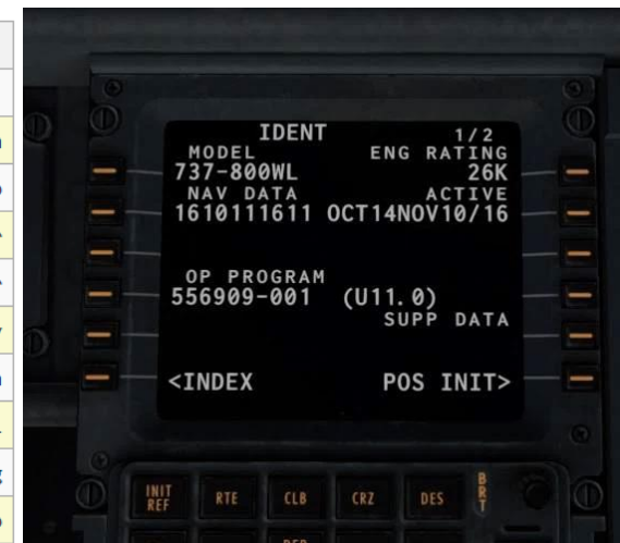
Modern FMS installed on a 737-800WL
