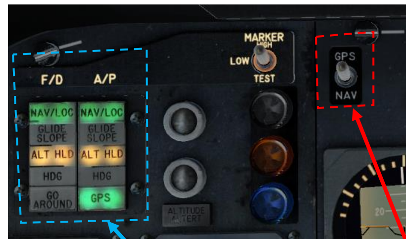
APD (Approach Progress Display) for Autopilot (A/P) and Flight Director (F/D)
