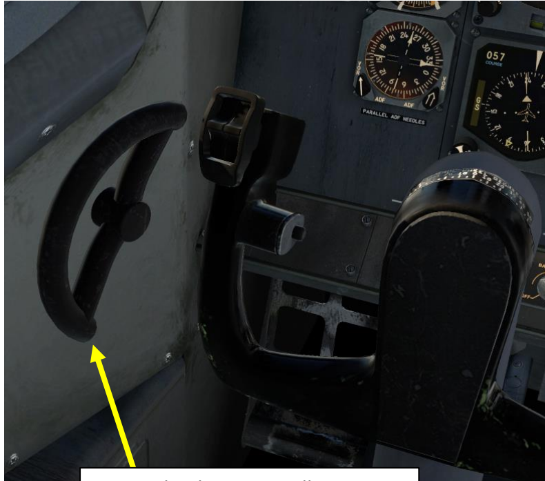
Nose Wheel Steering Tiller (used to steer aircraft on the ground)
