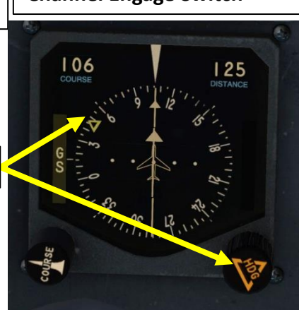
Heading Bug (HEADING SELECT)
